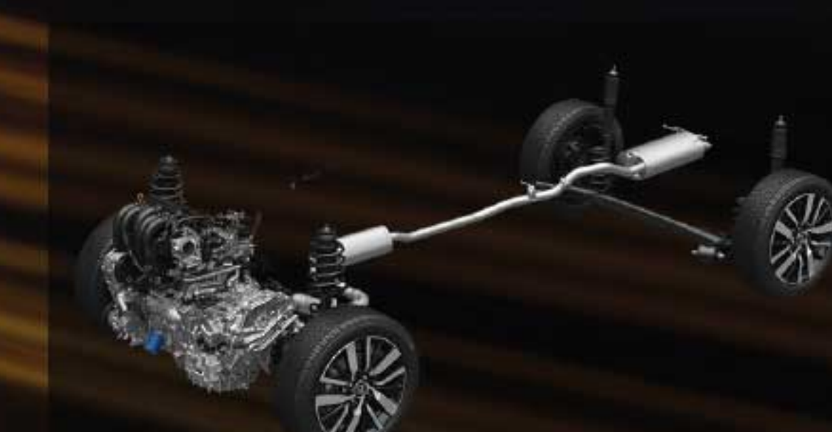
MacPherson Strut & H-Shape Torsion Beam Suspension
